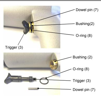
Replace and/or remove the spacer ring: to do this the gun needs to be partially disassembled.
